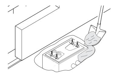
Remove the nuts from the screws.
