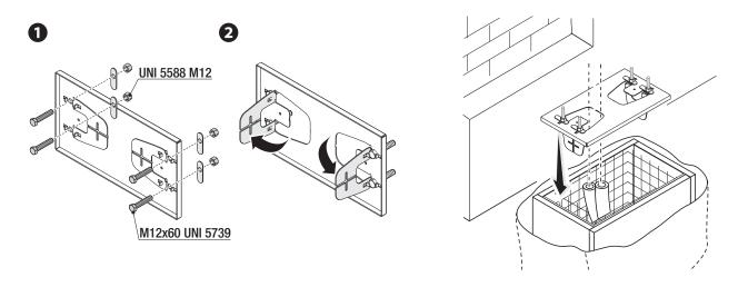
Position the anchoring plate, taking note of the measurements shown in the drawing.
